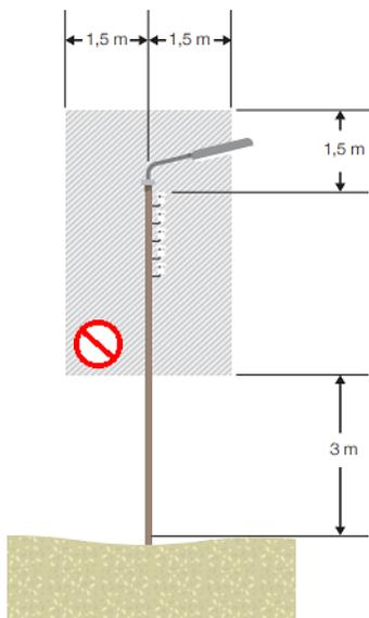
\* In the case of low-voltage overhead lines, work can be done above the masts by observing a safety distance of 1.5 m. / 5 ft.
