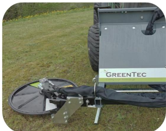
FOX Multi Carrier mounted with RI Barrier Mower in working position. The attachment tool can be further extended in reach using the Multi Carrier's arm system.
