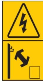
The higher the voltage, the greater the distance required between the power lines and the machinery! When in doubt – always contact the local power company for safety instructions!
