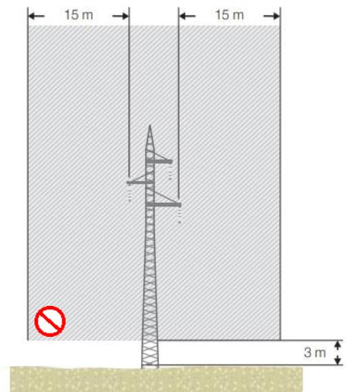
\* At a higher voltage than +400 kV: Safety distance must be determined by the network owner/operating manager or registered professional engineer.
