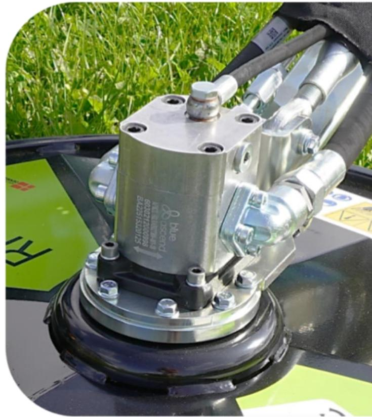
Hydraulic gear motor
