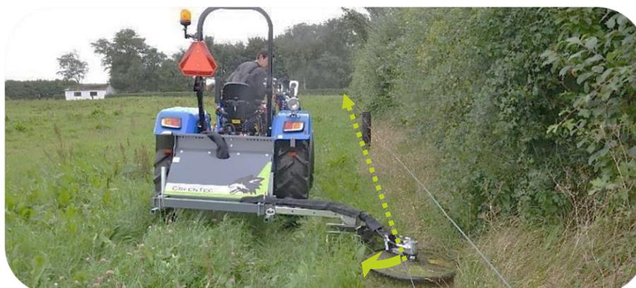
6. The forward speed when using the RI Barrier Mower must be max. 3-4 km/h (1.86-2.49 mph) and must always be adjusted so that the cutting result is optimal.
