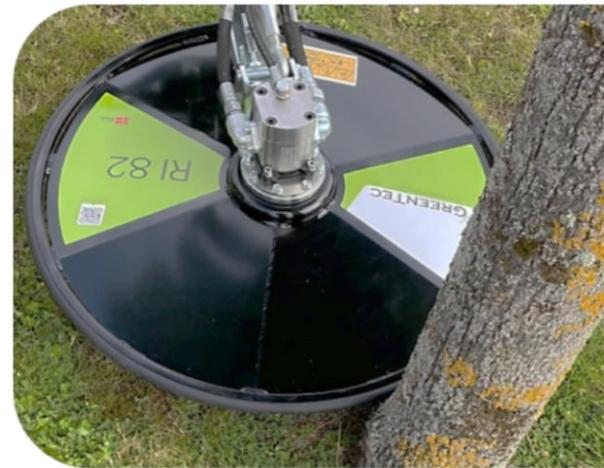
Rubber protection around cutting head
