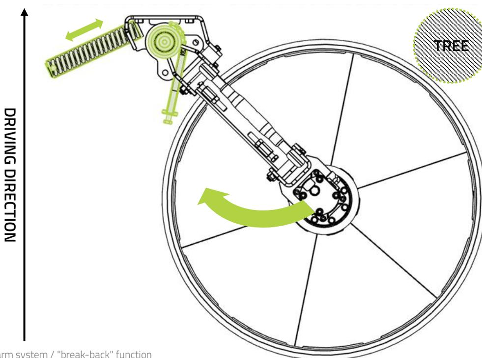
Function of spring-loaded arm system / "break-back" function
