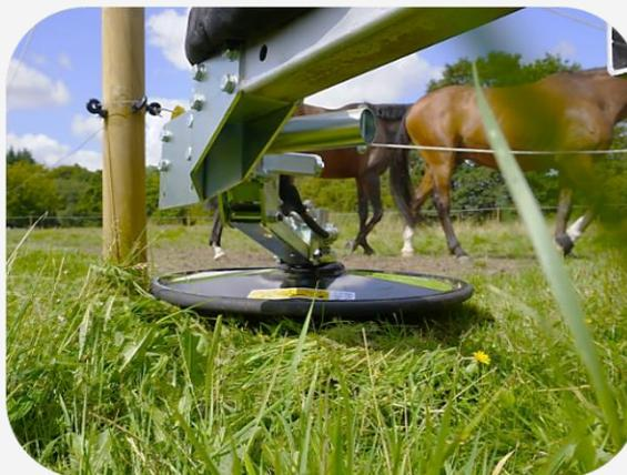
5. The direction of travel with the RI Barrier Mower must take place forward and must follow the contour of the ground and/or the line of the "fence".
