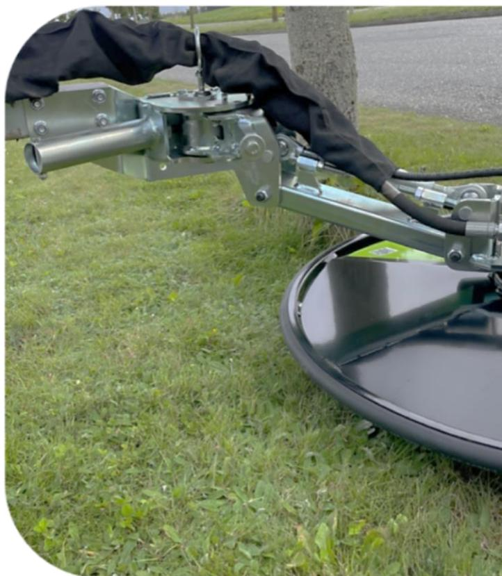
Spring-loaded arm system / "break-back" function
