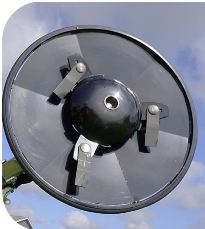
Blade rotor with hardened steel blades
