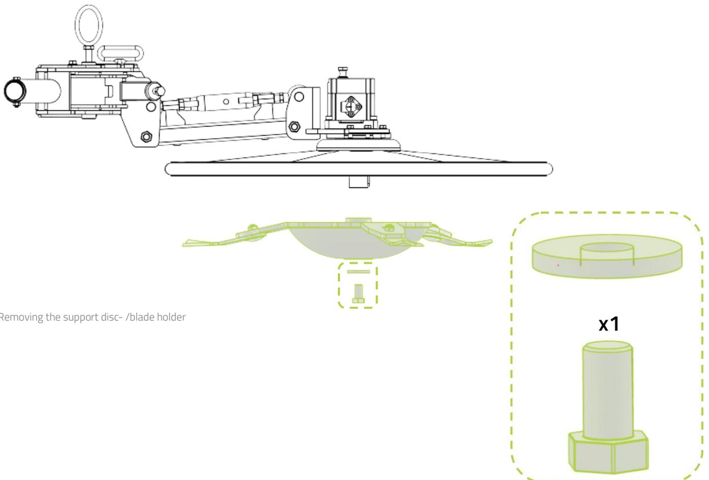
Removing the support disc- /blade holder
