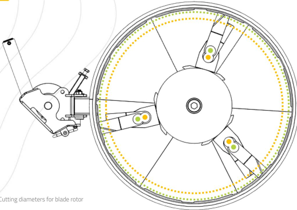
Cutting diameters for blade rotor
