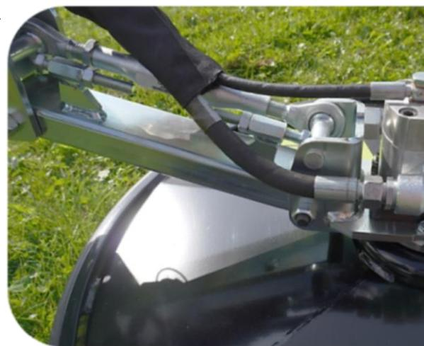
Adjustable suspension on RI Barrier Mower
