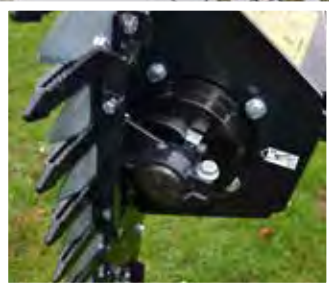
HD PLANETARY GEARBOX WITH CAST IRON ENGINE
