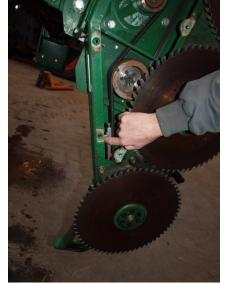
Remove cap. See adjustment bolt Loosen 3 bolts. Twist tensioner
