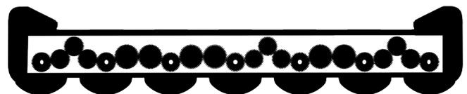
The specially ground surface of the gears submerged in gear oil ensures smooth running. This reduces the noise level considerably.
