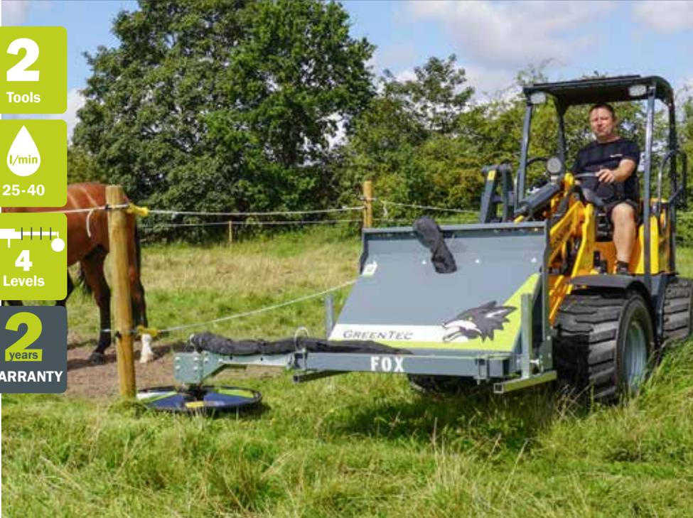
The Multi Carrier FOX is specially developed to carry our Barrier Mower RI 60 & 82. The FOX has many mounting options as it can be either front or rear mounted on tractors through category 1 or 2. The Multi Carrier FOX can also be front mounted on loaders. All that is required is an oil flow of 25 or 40 liters per minute.
